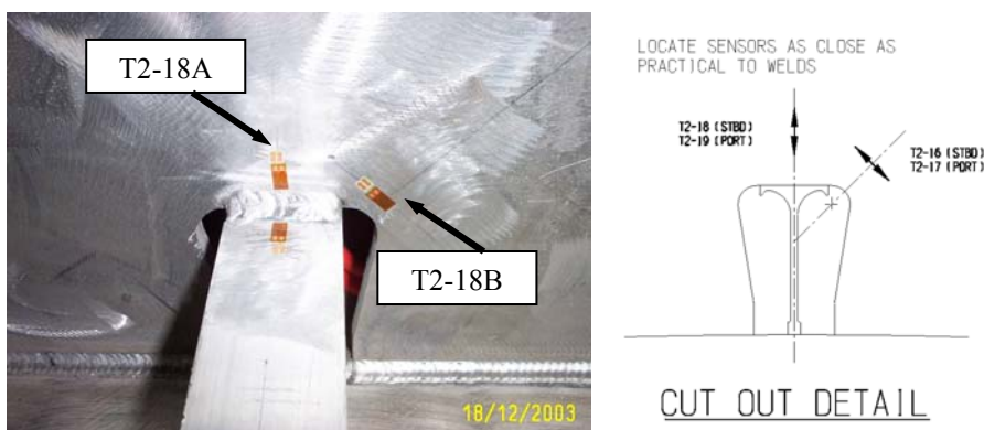
Fig. 2: Examples of local high stress T2 A-B pair strain gages
